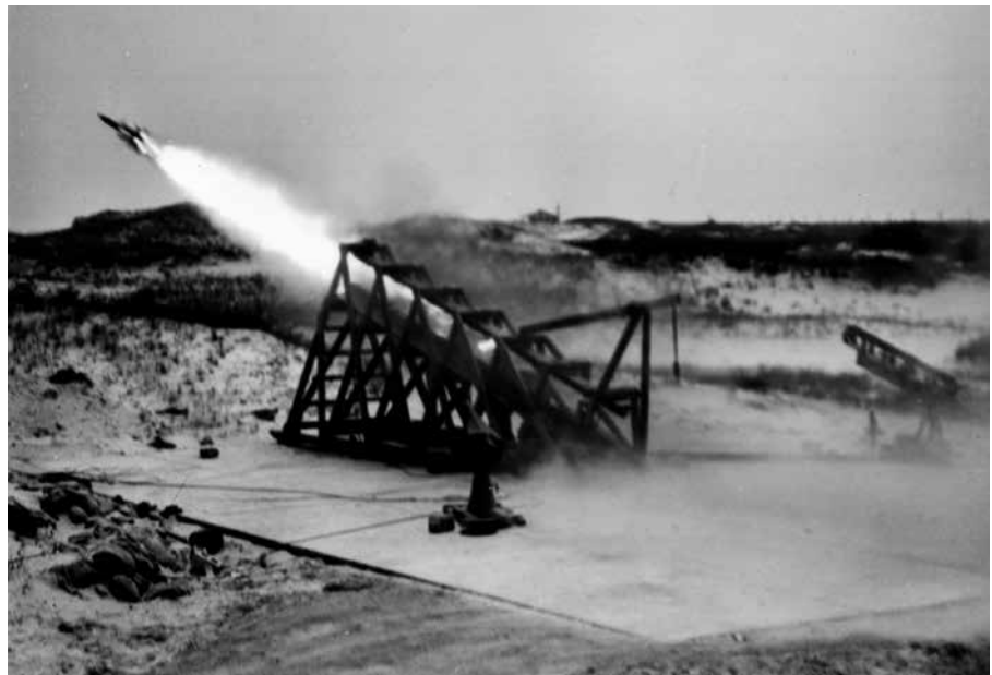
The "Flying Stovepipe" fires away from the Island Beach launcher. Fashioned from the exhaust pipe of a Thunderbolt fighter plane, this six-inch diameter missile attained a supersonic speed of 1,200 miles-per-hour on June 13, 1945.
